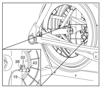
Then, plug in the power cord, press the power switch, and rock the Pulley (19) forward and backward just enough that the Magnet (43) passes the Reed Switch (38) repeatedly. Repeat these actions until the console displays correct feedback.
