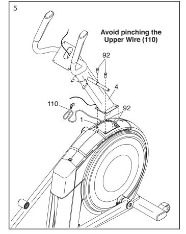
Locate the wire tie (A) in the lower end of the Upright (4). Tie the wire tie to the Upper Wire (110) as shown. Then, pull the upper end of the wire tie until the Upper Wire is routed through the Upright.
