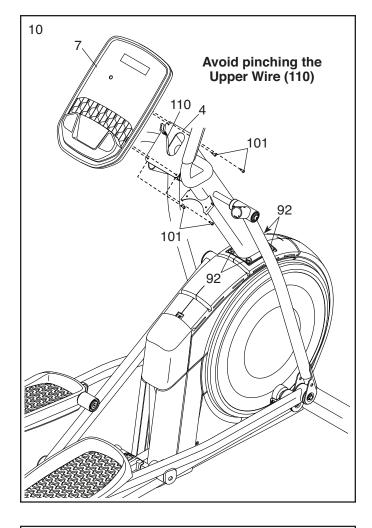
Orient the Rear Console Cover (80) as shown, and attach it to the Upright (4) with two M4 x 16mm Screws (101).
