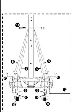
As shown on above picture, insert wheel shaft (10) into wheel (9), base (5) and wheel bracket (26) one by one.
