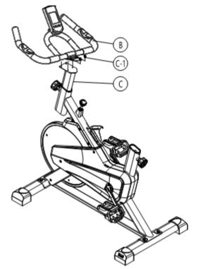
**Step 5.** Take out the monitor A# and phone holder B-3#. Install as shown in the pictures below: Buckle the phone holder B-3# and monitor A# onto the front handlebar B# with the arrow showing direction below. Insert the communication wires into the sensor slots on the back of the monitor.Insert the handle pulse wires B-6# into the PULSE slots on the back of the monitor.
