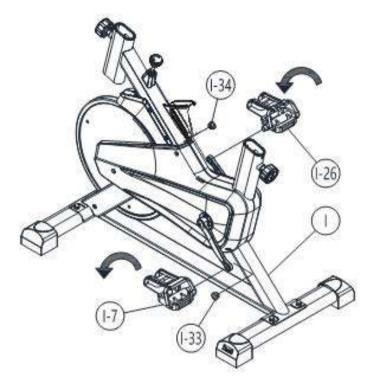
**Step 3.** Take out the Handlebar Post C#. Loose the Pull pin knob I-3#, and insert the handlebar post C# into the frame I#. Adjust the height of the handlebar post according to user's height and use the pull pin knob I-3# to lock it.
