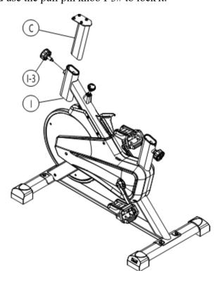
**Step 4.** Take out the Front Handlebar B# and install as shown in the figure below: Use Allen key K-4# to remove the pre-assembled Hexagon socket head cap screw. Install the front handlebar B# and align it with the handlebar post C# and use the Allen key K-4 and screw C-1 to secure it.
