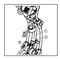
Next, push the upright (C) in the opposite direction slightly, lift the latch (D), and then lower the upright to the folded position. Hold the upright in one of the indicated locations (E) while you lower the upright; do not hold the upper body arms.
