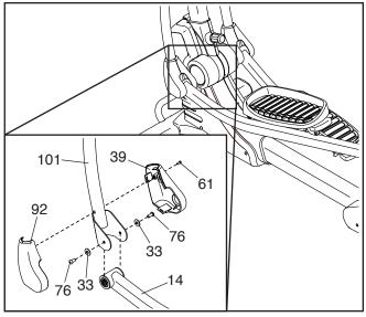
Then, remove the two M8 x 15mm Hex Screws (76) and the two M8 Washers (33) from the Left Upper Body Leg (101) and the Left Pedal Arm (14).
