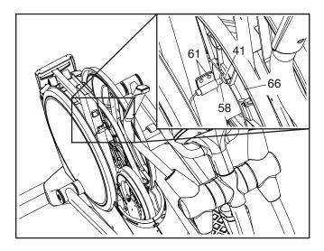
Plug in the power adapter, press the power switch to the reset position, and rotate the Pulley (66) for a moment. Repeat these actions until the console displays correct feedback.
