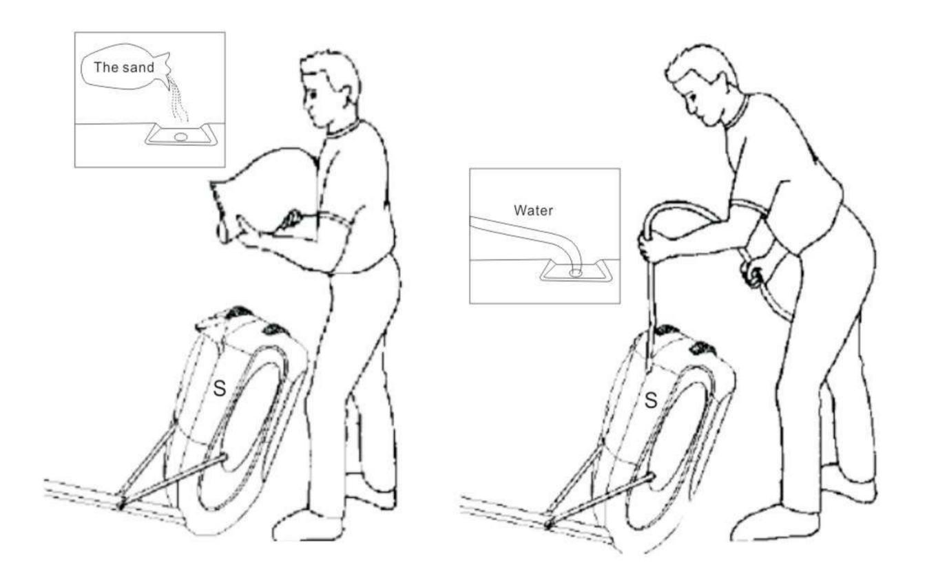
Filling the Base(S)with water or sand to keep steady.
