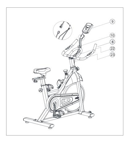
The Monitor Holder (10) is pulled and fixed on the Handle Frame (6) with the Self tapping screw (24) and tightened with the inner hexagonal wrench (27).
