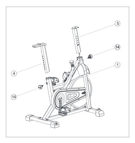
The Saddle Post (4) is inserted into the Main Body (1), and the Adjusting knob (14) is pulled out so that the Adjusting knob (14) is automatically inserted into the corresponding hole of the Saddle Post (4).
