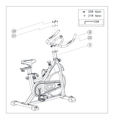
The handle frame (6) is fixed on the handle post (5) with the spring washer (21) and the round head bolt (20) and tightened with the Allen wrench (25).
