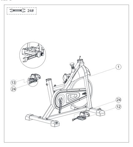
Install the right pedal (12) with the R mark displayed onto The Main Body (1) and fix it with an open wrench (24). Note: tighten it clockwise.
