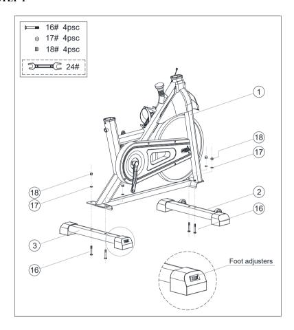
The Front Stabilizer (2) is fixed on the Main Body (1) with Carriage Bolts (16), Flat washers (17) and cover nuts (18), and fixed with the open wrench (25). Note: the wheels that can be used for transportation on the Front Stabilizer (2) are facing forward, as shown.
