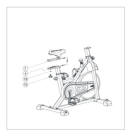
The seat adjustment frame (7) is installed on the seat post (4) and is fixed with a flat washer (19) and an adjusting nut (15).
